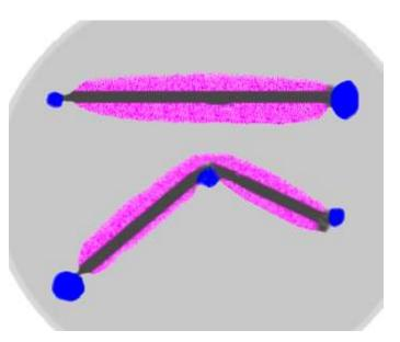
The illustration above shows 2 nails immersed in an agar gel containing phenolphthalein and  $[Fe(CN)_6]^{3-}$ . The nails can be seen to have started to corrode since the Prussian blue formation indicates the formation of Fe(II) (the Anodic sites which correspond to the end of the nails and the bend in the middle). The phenolphthalein (change to pink in presence of base) shows the build up of OH<sup>-</sup> and shows that essentially the whole length of the nail is acting as the cathode.
