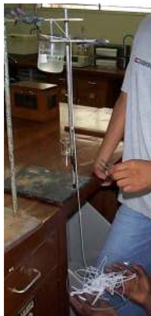
Preparation of thread of Nylon 6 10 in the Physical Chemistry Laboratory
