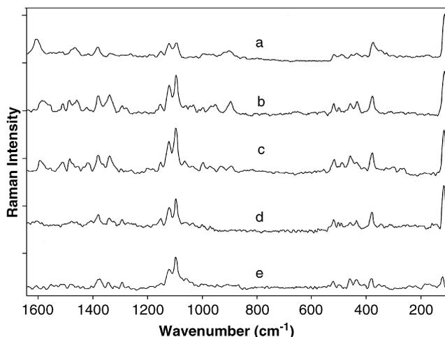
**Figure 7.** FT-Raman spectral stack plot of artificially aged new sailcloth specimens labelled (a)–(e), representing consecutively the non-aged, brine treated, brine and light treated, brine, light and heat treated and brine, light, heat and light treated specimens, respectively. The details of the ageing cycles are provided in the text.
